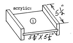
(a) For the Oersted effect, drill a single 1/16" (5/64") hole in the center of the acrylic on a drill press (if possible) for the #16 wire. Also, drill holes through the plywood to receive the wire (see diagram). Bend and straighten the wire while pushing it through the holes; connect the DC power supply with alligator clips.
