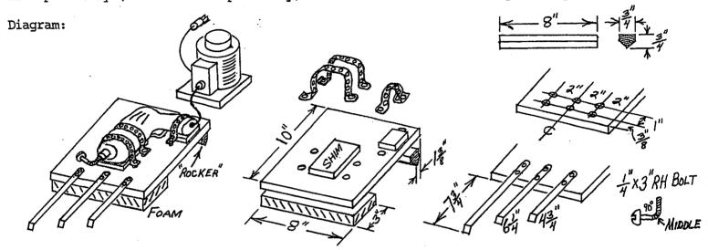
Addendum: Now that you have a good vibrating platform, you can extend its use to replicating a a quality shaker table I first saw at N.Y.U. in the 1960's. It was probably used to study resonance and standing waves in skyscrapers during earthquakes.
