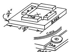
3/16". Place solenoid on end in center of base; mark position of tabs along the edges, apply glue (Elmer's?), and nail down with brads. With 4 washers and #8 x 3/4" woodscrews, position washers so they overlap the edge of the solenoid's base. Mark and drill screw holes. Screw down the solenoid in place; everything should fit tight.
