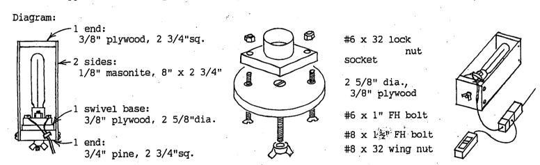
Materials: 1 med. base #9063 Leviton pony cleat lampholder, 1 #TBI03 Leviton plug-in lamp dimmer switch, 30" #18 lamp cord wire, 1 male plug, 3 FH bolts, 2 lock nuts, 1 wing nut, 4 #6 x 5/8" PH screws, 3/4" pine board or plywood, 3/8" plywood, wire restraint (staple?)
