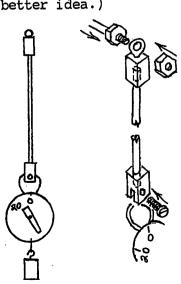
Based on your resources, you must decide how you want to mount the pendulum for display. Remember, a swinging, 1 kg, hooked mass will want to "sway" the pivot point which needs to be kept motionless (rigid) for best results. A plan of my "rigid" stand in included; if you have a better plan, use it.
