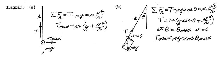
In (a) the gravitational force component and centripetal effect are at their maxima. In (b) the component force of mg along the string is reduced by  $\cos\theta$  and the centripetal effect drops to zero. Of course, in every position between (a) and (b), the tension will be changing between the maximum of (a) and the minimum of (b).
