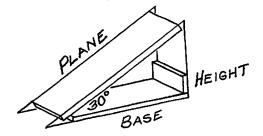
Suggested dimensions: 1/8" masonite sides: base  $- \sim 17$  11/16 in., height  $- 10\frac{1}{4}$  in., plane (hybtenuse)  $- 20\frac{1}{2}$  in.
