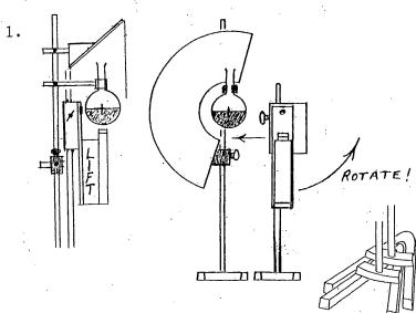
The principle: With a laser beam beneath the center of a half-filled flask of water aimed straight up, the beam will travel straight up through the glass bottom and the water, and then straight up the neck. (Minor surface reflections will occur, of course.)
