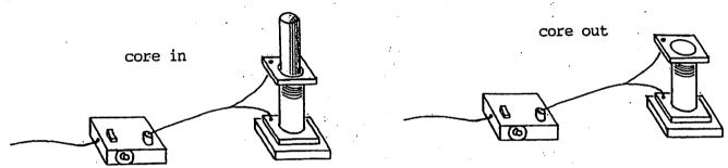
Begin the demonstration with the iron core all the way in the solenoid as in the left diagram. Using the switch box, turn on the circuit. With the "choke" (iron core) in, the self-inductance (impedence) is high enough to keep the current down (choked) to a level that the circuit can handle. Don't let this circuit operate for more than 30 sec.; 20 sec. might be enough because of coil heating. Turn off the circuit, and let the coil cool down, if warm, for a minute or two.
