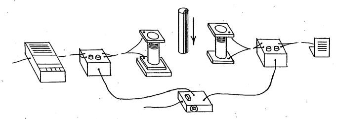
Begin simply with a tape player and a patch cord from its earphone jack to the primary coil (the "broadcast antenna"). Leave out the amplifiers for the moment. From the secondary coil (the "receiving antenna"), patch a cord directly to the speaker. You are about to demonstrate "near-field" radio wave transmission in its simplest form. With the coils close together, side by side, play the tape and listen to the speaker; the sound should be very faint.
