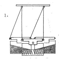
Now rearrange the two threads by putting their tops together in just one screw eye. Swing the apparatus again. A different result! This time the container and the fluid are swinging in unison, thus, no "slope" (incline) is evident. The acceleration present is centripetal acceleration or toward the center of rotation, perpendicular to the apparatus (2.).
