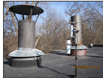
Figure 5. A picture of the cascade impactor on the roof of the crematorium Vale Cemetery in Schenectady, NY.
