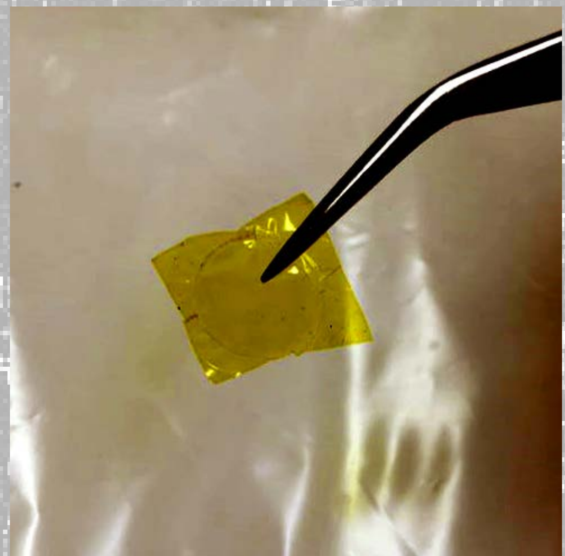
Figure 1: A photo of a square of 7.5 micron thick Kapton foil used for the window of the external beam facility.
