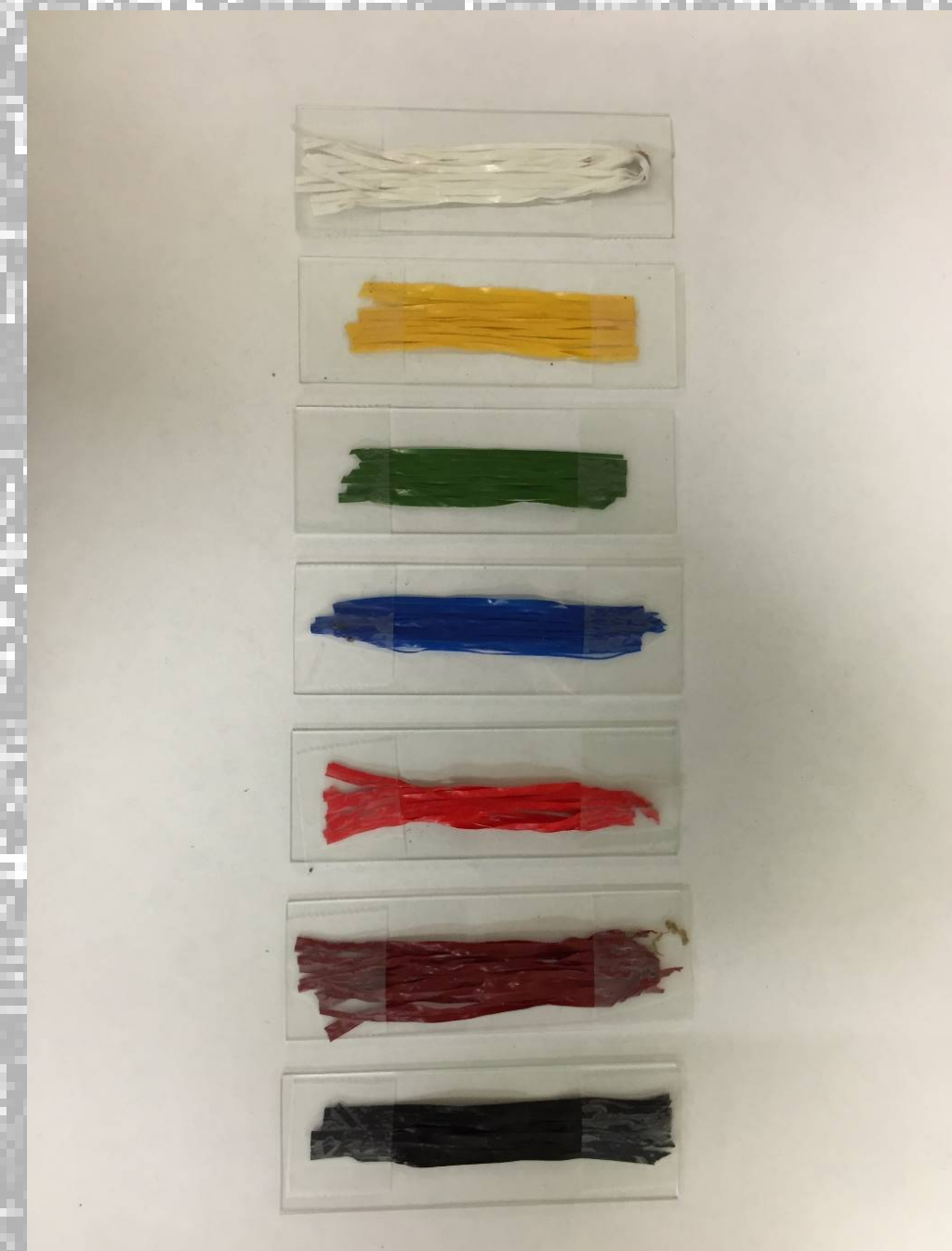
Figure 5: A photo of the different color turf blades coated in gold and palladium to keep them from charging when the samples were bombarded with the proton beam.
