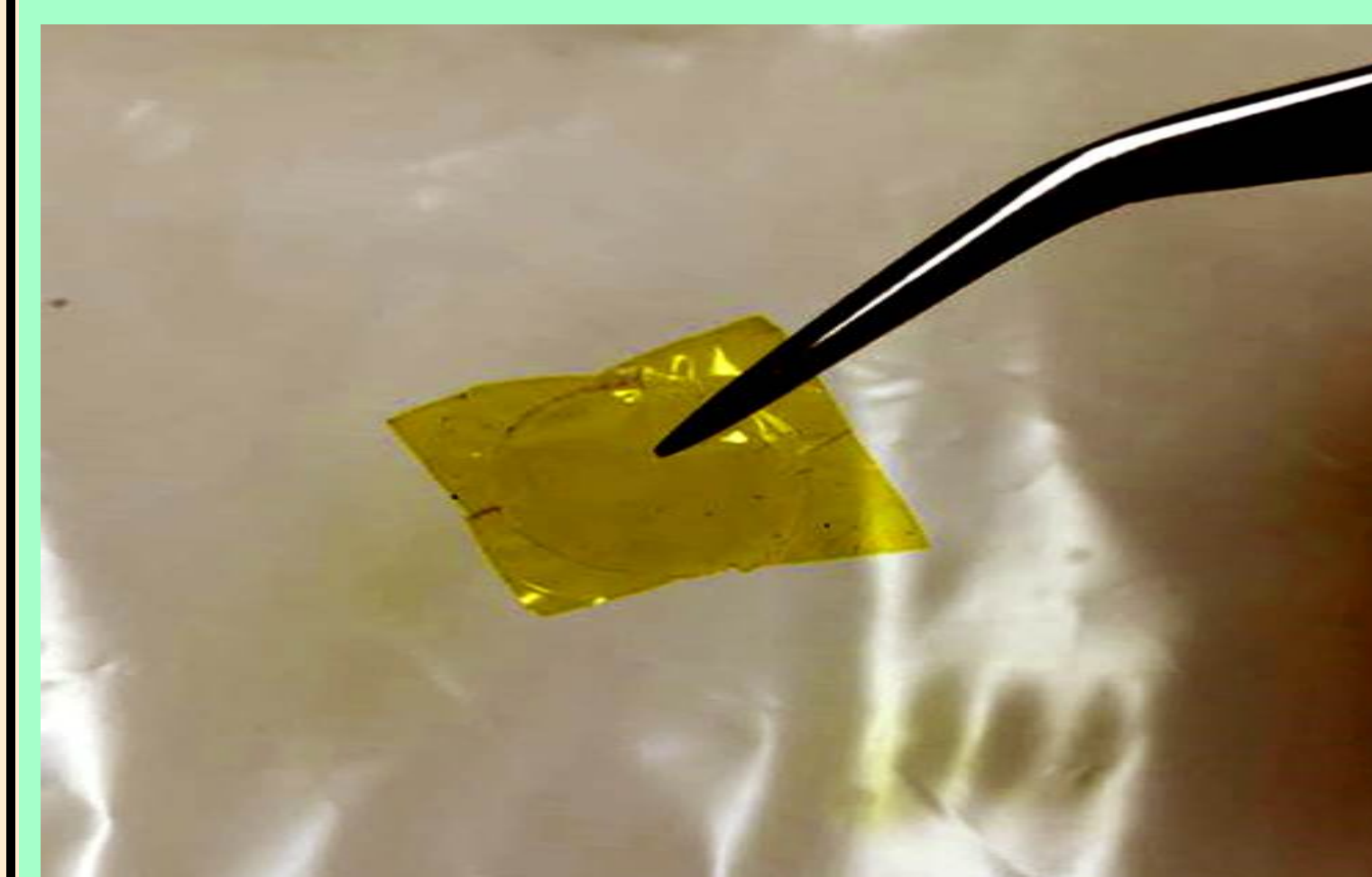
Figure 4: A photograph of the 7.5- \mu\text{m} thick Kapton foil used for the vacuum window.
