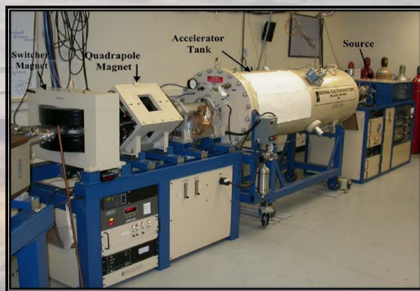
Figure 2: A photograph of the UCIBAL's 1.1 MV tandem electrostatic accelerator showing the main components. The protons are generated in the Source and accelerated through the accelerator tank to a final energy of 2.2 MeV. They are focused and steered toward the target using the Quadrupole and Steering magnets respectively.
