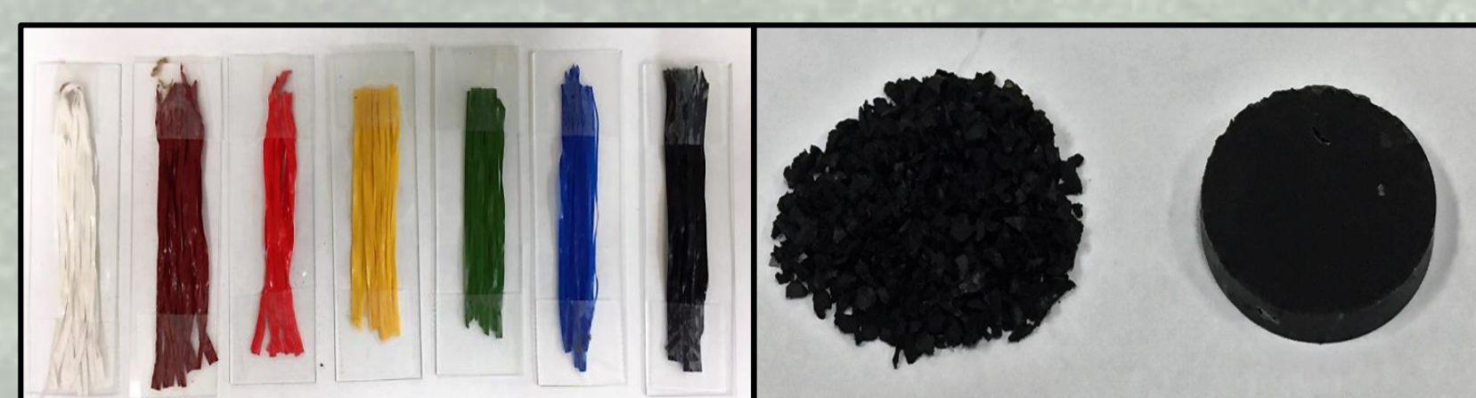
Figure 2 A photograph of some artificial turf blades before being coated with Al on the left. On the right, 1g of loose crumb rubber infill and 1g of infill pressed into a pellet with ~1g of epoxy.
