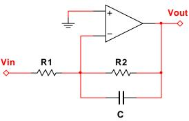
c) Let us assume that the circuit from Part (b) passes a signal frequency when  $|V_{OUT}/V_{IN}| > 0.9G_O$ . Suppose R1 = 1 kohm and R2 = 100 kohm. Assume the ECG signal has frequency content that spans from 1 to 30 Hz. What is the appropriate value for C in order to suppress noise? Choose a standard 10% capacitor value (see table on last page). Show all work!
