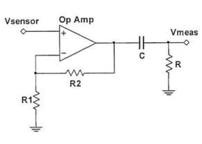
(d) We want to suppress signal frequencies below 10 Hz. Suppose a frequency is "rejected" if |V<sub>meas</sub>/V<sub>sensor</sub>| < 0.1G. Assuming R = 10 kohm, what is the appropriate value for capacitor C? Choose a standard 10% capacitor value (see table on last page). Show all work!
