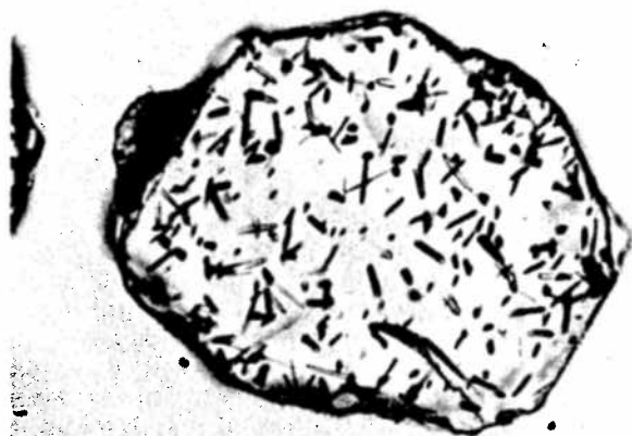
Figure D17 Photograph of fission tracks in a detrital apatite crystal from the mid-Cretaceous Jackass Mountain Formation, British Columbia. This apatite has a mid-Tertiary cooling age, so the strata were buried, heated, and then cooled in the Eocene. This apatite is about 150 \mu\text{m} across and horizontal tracks are about 12 \mu\text{m} long. This apatite crystal is mounted in epoxy, polished so an internal surface is exposed, and the chemically etched tracks are oriented in all directions, so some are short vertical track tips, while others are nearly horizontal and a full length can be seen. (Photo: J. I. Garver.)
