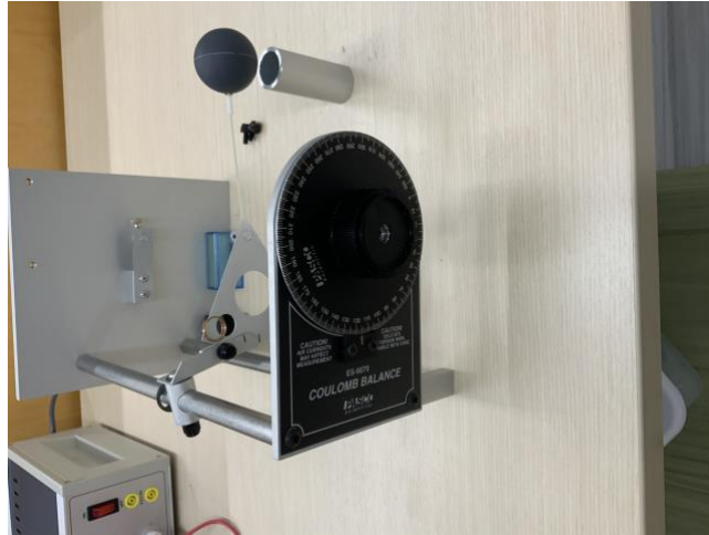
Figure 2: Torsion balance on its side with the slide assembly removed.
