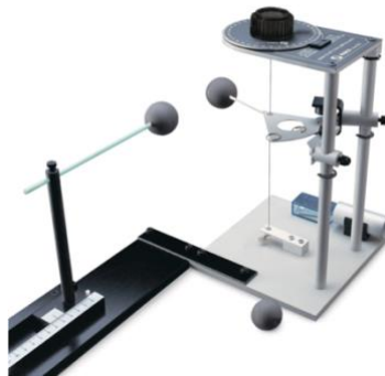
Figure 1: The Coulomb Balance apparatus ( https://www.pasco.com )
