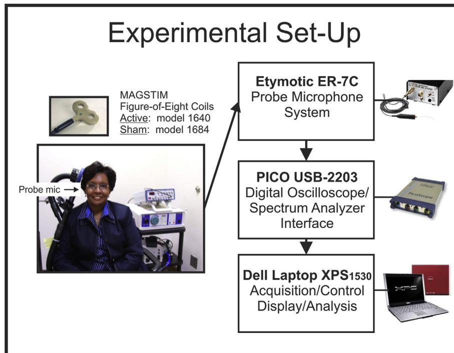
**Fig. 11.** Block diagram of the experimental set-up used to measure SPLs at the lateral surface of the tympanic membrane in the ear canal with a probe-microphone system in place.
