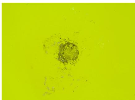
Figure 2. A microscopic image of an aerosol deposit on one of the Kapton impactation foils.
