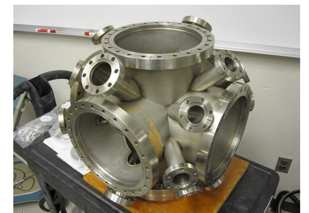
Figure 11: A photograph of the 10-inch, multi-way, Conflat cross that is the basis for the new scattering chamber at UCIBAL.
