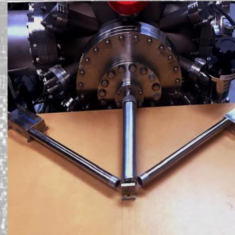
**Figure 8:** A setup of the beam with the x-ray and gamma ray detectors and sample. We place samples that we wish to analyze in front of the beam on a line drawn on the table. There are guides and markings on the table to help ensure that the sample and detectors are in the same place relative to the beam every time a test is run.
