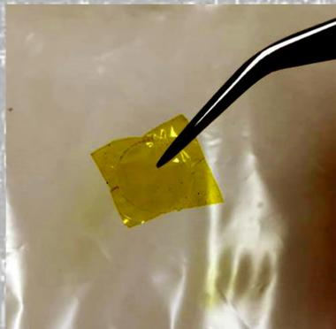
**Figure 1:** A photo of a square of 7.5 micron thick Kapton foil used for the window of the external beam facility. It was placed over the 1/4" diameter hole in the center of *Figure 2* underneath the plate that can be seen in the figure.
