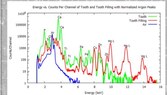
**Figure 10:** PIXE Spectra [3] of the tooth filling (red) shown in *Figure 9*, the tooth (green) also shown in *Figure 9*, and a run on just the air (blue). We normalized the argon peak of each spectra in order to fit it all to one plot.
