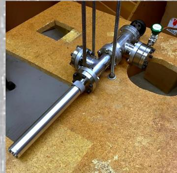
**Figure 3:** A picture of the test set-up of external beam facility. We attached a vacuum pump to test the window's ability to withstand vacuum.
