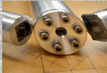
**Figure 4:** A close-up of the tip of the beam pipe and detectors when attached to the accelerator. They rest on a table marked at specific angles and distances to aid in the placement of samples and the detectors from run to run.
