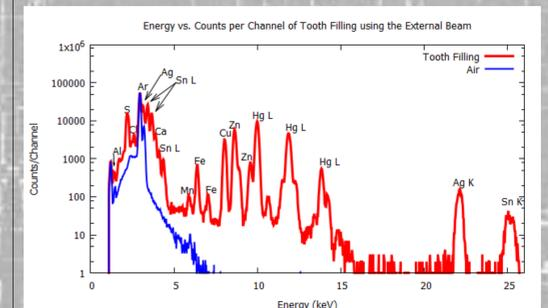
**Figure 11:** PIXE spectra [3] of the tooth filling shown in *Figure 9* and the air. As can be seen, this filling contains mercury, silver and tin.
