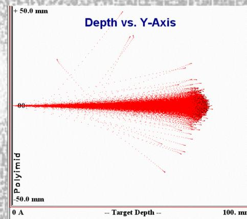
**Figure 7:** A TRIM simulation [2] of a 2.2MeV proton beam after it has traveled through a 7.5 micron thick Kapton foil and is moving through the air. This simulation models the divergence of the beam and demonstrates how much it spreads out as it travels through the air. According to this simulation the beam travels approximately 8 cm in the air before it is stopped, although we run on them. At this distance, the energy of the beam drops to about 1.7 MeV.
