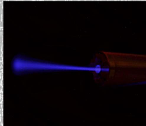
**Figure 6:** A photo of a 2.2 MeV proton beam in air coming out of the external beam facility to the right.
