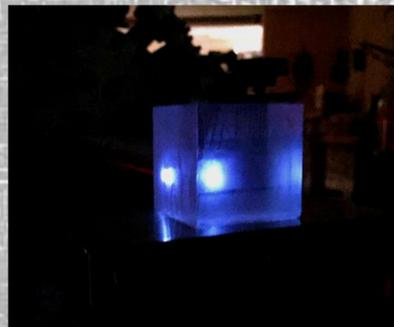
**Figure 5:** A photograph of the beam entering a block of plastic scintillator. When the proton beam passes through the block, it glows blue. This test allowed us to determine that the beam was aligned properly.
