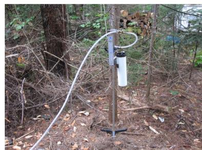
Figure 5: A photograph of the nine-stage impactor set up near Piseco Lake.
