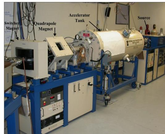
Figure 6: A photograph of the Union College Pelletron Accelerator.
