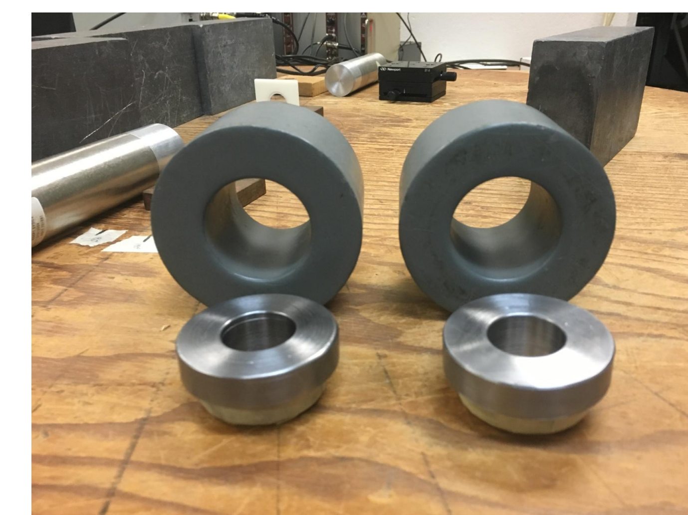
Figure 10: Photograph of the lead collimators for the detectors.
