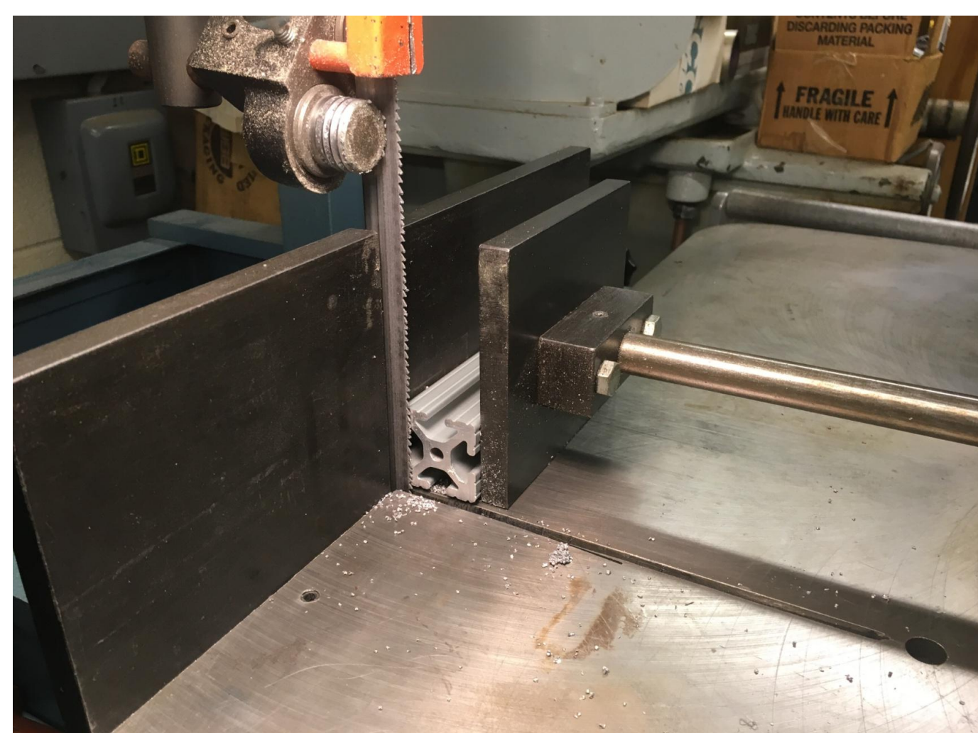
Figure 2: Photograph of a leg of the stationary arm being cut.
