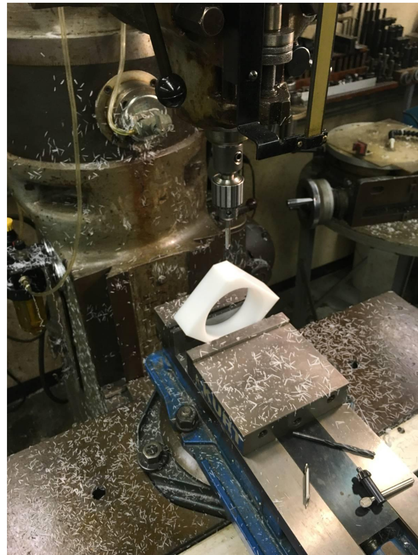
Figure 3: Photograph of a detector holder body being cut.
