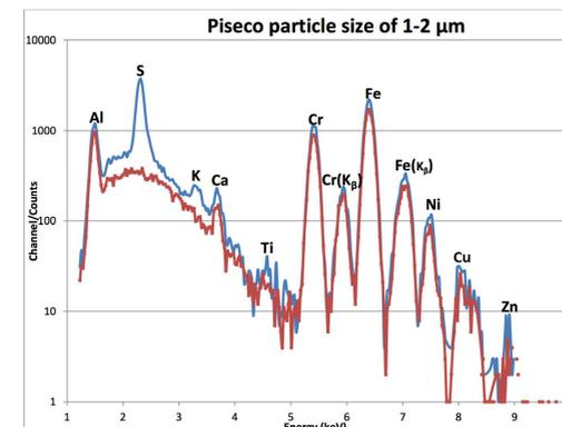
Figure 9: Comparison of PIXE spectra taken on an impacted Kapton foil with particulate matter between 1-2  $\mu$ m (blue) and a blank Kapton foil (red).
