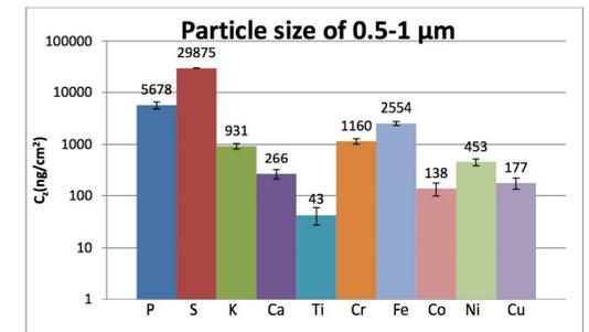
Figure 10: A bar graph of concentration in ng/cm<sup>2</sup> vs. element for particulate matter of 0.5-1  $\mu$ m in size.
