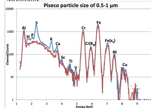
Figure 8: Comparison of PIXE spectra taken on impacted Kapton foils (blue) for particle size of 0.5-1  $\mu$ m and a blank Kapton foil (red).
