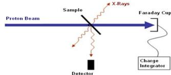
Figure 1: A schematic of a basic PIXE experimental setup for thin targets
