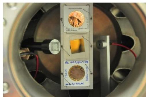
Figure 7: A photograph of the inside of the scattering chamber showing the target ladder (center), the X-ray detector (left), and a charged particle detector (right).
