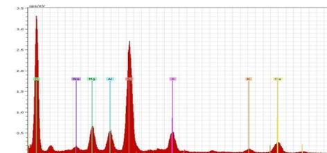
Figure 10: An EDX-spectrum taken on particle 1 in the SEM image shown in Figure 9.
