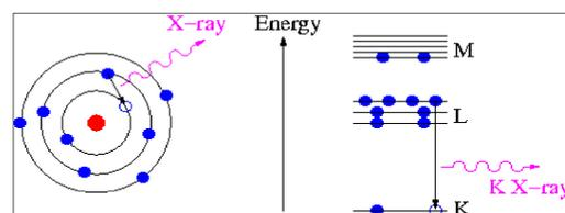
Figure 3: An X-ray is emitted when the void is filled by an outer shell electron.
