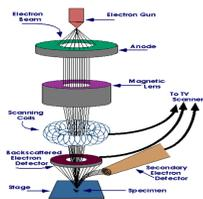
Figure 1: A schematic diagram of the scanning electron microscope.[2]
