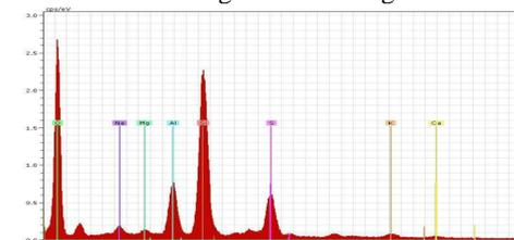
Figure 11: An EDX-spectrum taken on particle 4 in the SEM image shown in Figure 9.
