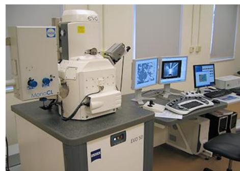
Figure 6: A photograph of the Union College Scanning Electron Microscope.
