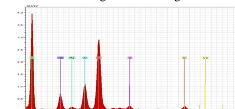
Figure 14: An EDX-spectrum taken on particle 5 in the SEM image shown in Figure 12.
