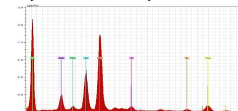
Figure 13: An EDX-spectrum taken on particle 2 in the SEM image shown in Figure 12.
