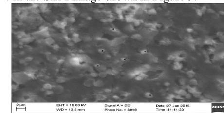
Figure 12: An SEM micrograph of the stage 2 sample with six individual particles labeled.
