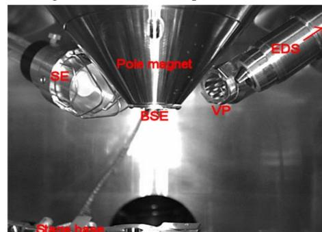
Figure 7: A photograph of the inside structure of the SEM.
