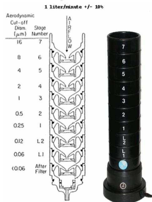
Figure 4: A schematic and photograph of the nine stage cascade impactor [1].
