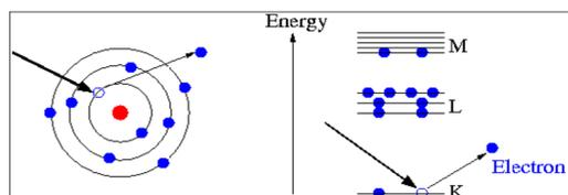
Figure 2: The ejection of an inner shell electron by an electron.
