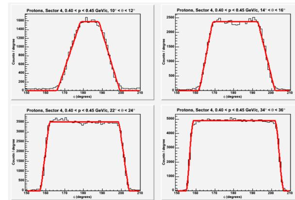
Figure 3: Azimuthal angle distributions for protons detected in Sector 4 with momenta between 0.40 and 0.45 GeV/c for several different bins in scattering angle. The trapezoidal fits are shown in red. The  $\phi$  range between the top corners of each trapezoid represents the region of flat acceptance for that bin.
