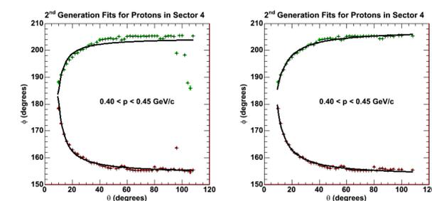
Figure 4: Fits of the  $\phi$  position of the corners of the trapezoids as a function of scattering angle for protons in Sector 4 with momenta between 0.40 and 0.45 GeV/c. The left and right panels show the fits before and after a few outlying points at large scattering angle were removed.
