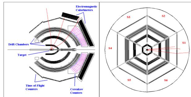
Figure 2: Schematic diagrams of the CEBAF Large Acceptance Spectrometer in Hall B at Jefferson Lab. The left (right) panel shows a slice parallel (perpendicular) to the beam axis. The red curves are simulated proton tracks [2].
